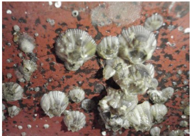
Photo 2: Barnacles – medium calcareous fouling
