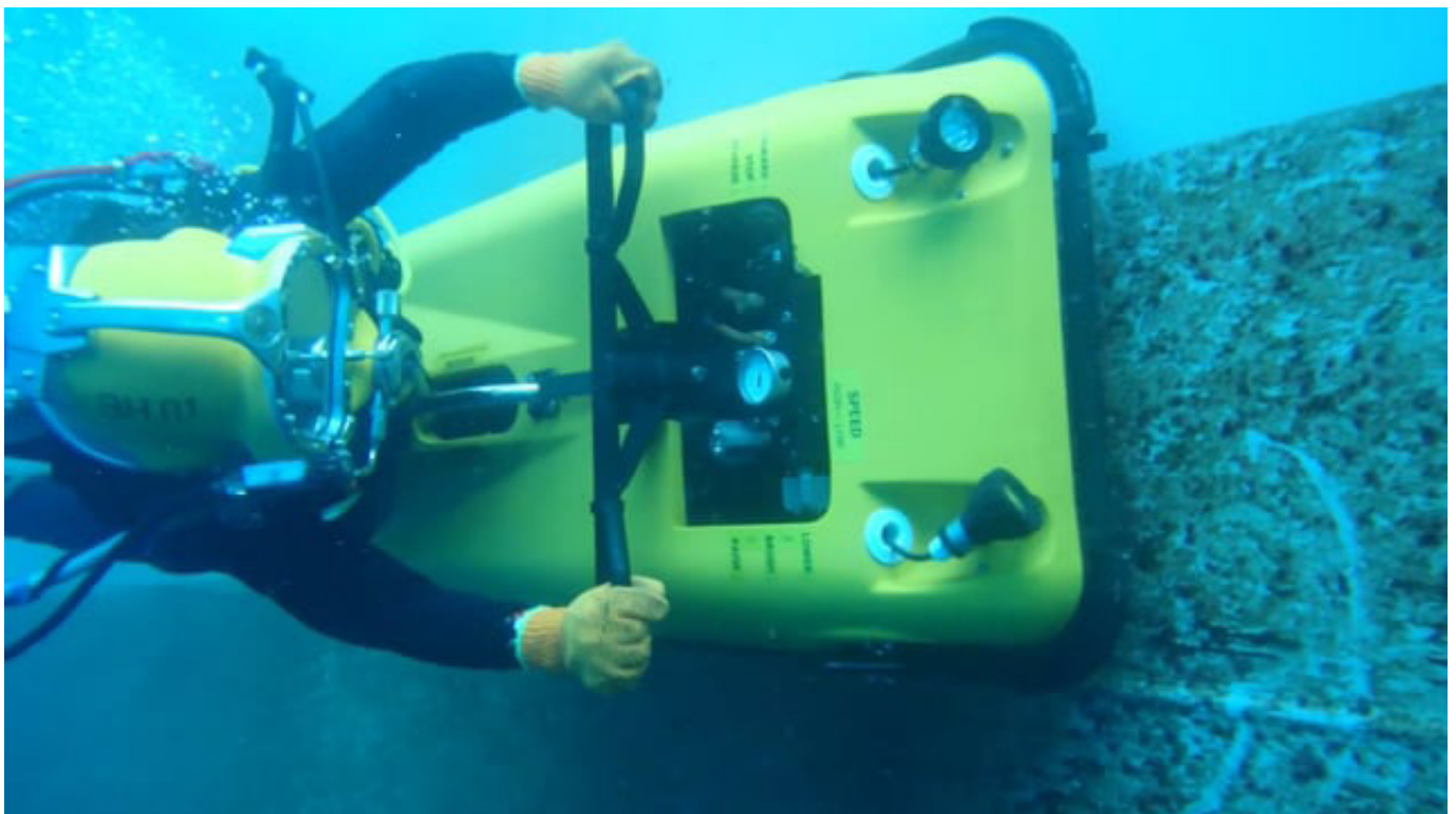
Photo 4: Diver-operated cleaning cart.
